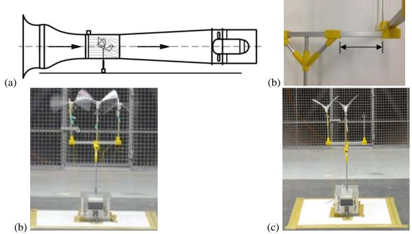
Figure 3: Setup of the Wind Tunnel Test (a) Schematic; (b) Definition of Distance between Ornithopters; (c) Tri-flapper Case; (d) Bi-flapper Case
