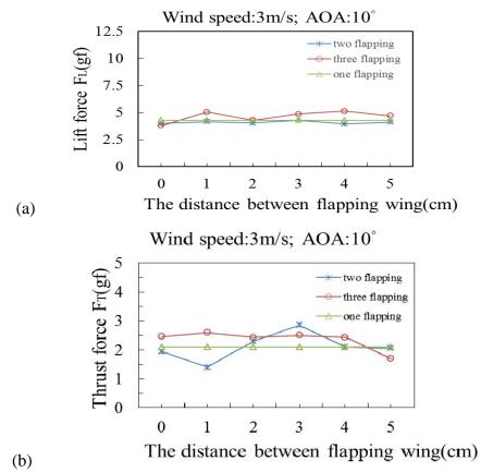
Figure 4: The Best Case of Wind Tunnel Test (U=3m/s;AOA=10°) (a) Lift; (b) Net Thrust vs. distance between ornithopters
